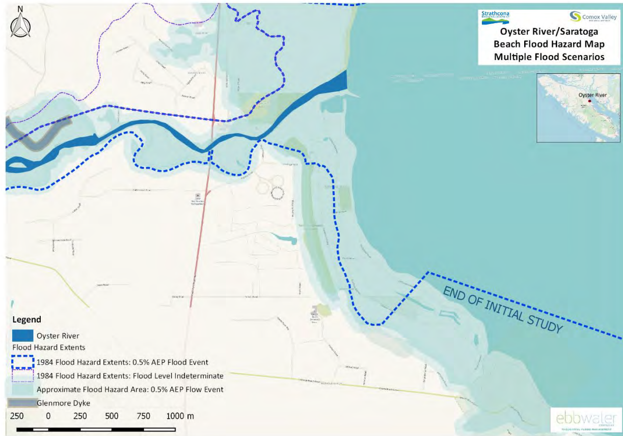
Figure 4: Map of Oyster River/Saratoga Beach with the extents from the 1984 model and updated high level modelling
